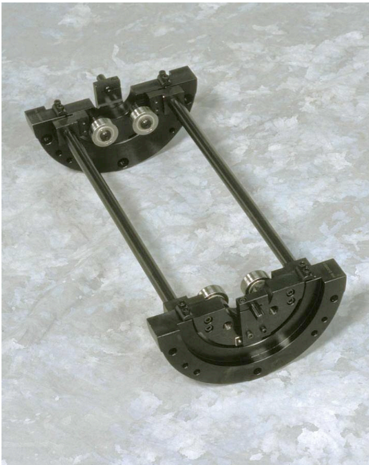
Balancing fixture for a 50-pound Class 100 / Class 300 SAE Proving Rotor. Related balancing tooling such as this fixture also requires periodic inspection and recertification.
